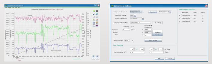
Through SUTO software S4A recordings are downloaded to the PC via USB or Ethernet port. The basic analysis can be done in S4A.
