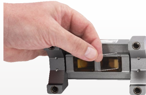
Placing the couplant pads before installation on the transducer surface
