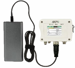
S461 powered by power bank with connection cable.
