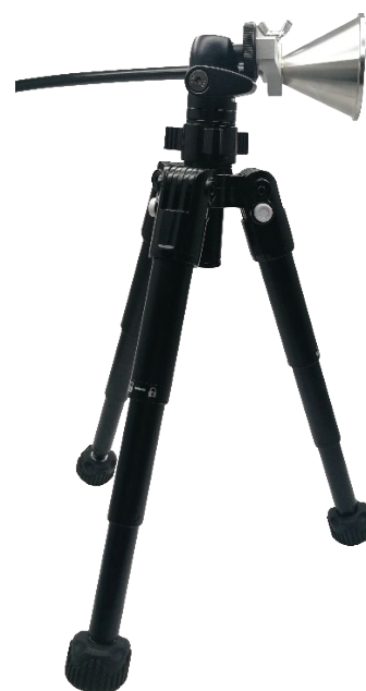
Isokinetic sampler with stand and hose
