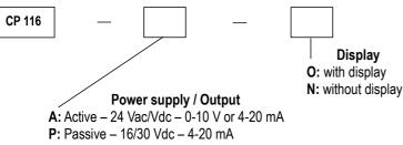
Example: CP 116 - PO Transmitter of atmospheric pressure, passive transmitter 16/30 Vdc, with display
