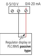
Connection of output in voltage 0-10 V:
