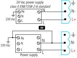
> For transmitters with 100-240 Vac power supply:
