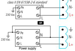
For transmitters with 100-240 Vac power supply:
