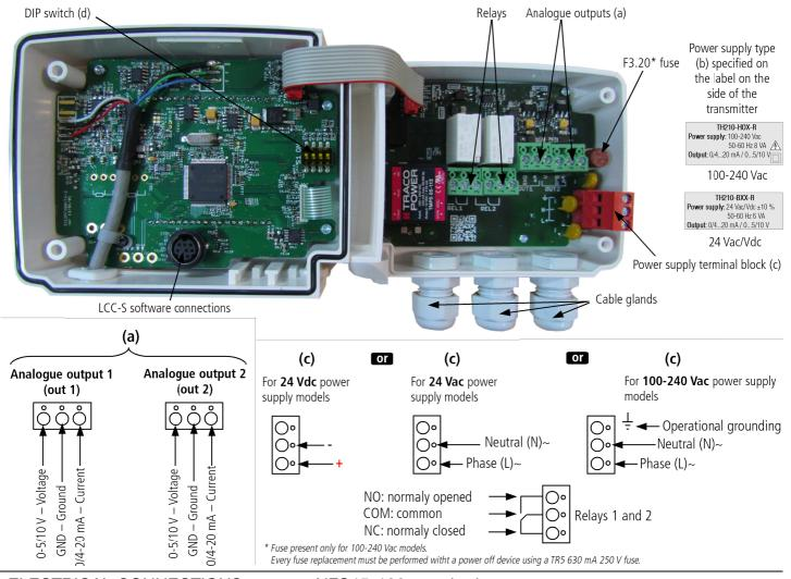
This connection must be made by a formed and qualified technician. To make the connection, the transmitter must not be energized. Before making the connection, you must first check the power supply indicated on the transmitter board (see (b) on "Connections" part).
