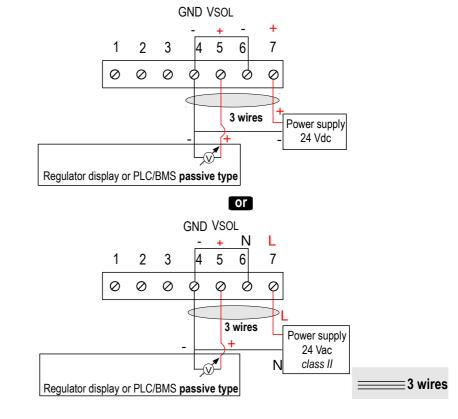
For **CR110-PO** models with 4-20 mA output – **passive**:
