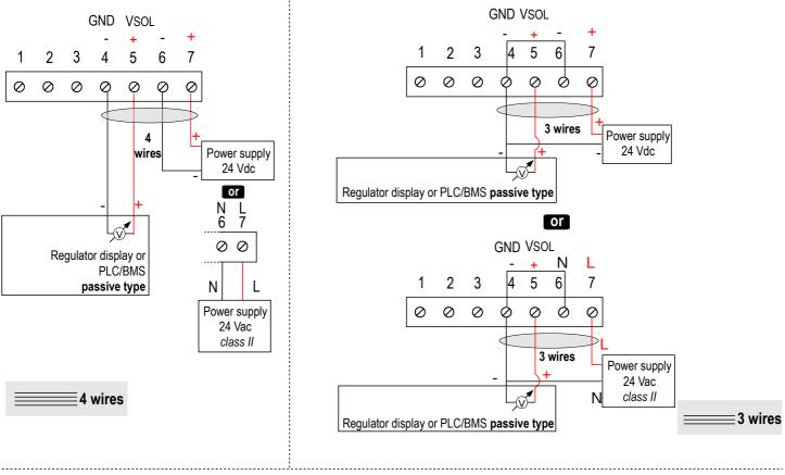
For CR110-PO models with 4-20 mA output – passive:
