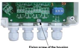
Fixing screw of the housing
